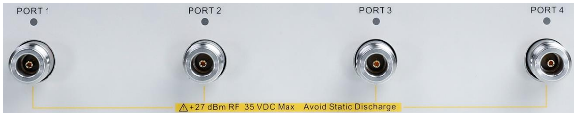
Figure 1-6 Front panel RF connectors (4-port VNA)
