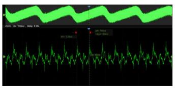
Using hardware-based Zoom technique and record length of up to 500 Mpts, users can select a slower timebase without compromising the sample rate, and then quickly zoom in to focus on the area of interest
