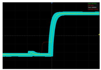
The oscilloscope utilizes a hardware-based Mask Test function, performing up to 18,000 Pass / Fail decisions each second. It is easy to generate user-defined test templates to provide trace mask comparisons, making it suitable for long-term signal monitoring or automated production line testing
