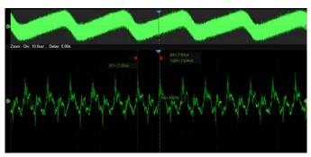
Using hardware-based Zoom technique and record length of up to 200 Mpts, users can select a slower timebase without compromising the sample rate, and then quickly zoom in to focus on the area of interest
